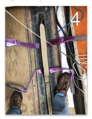
Back to <u>Harbor Freight!</u> I grabbed a chain hoist and used a laughably heavier-than-needed beam I made for something else to lift the centerboard (5-7).
