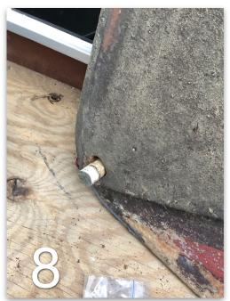
Once on the cabin sole, the pivot pin (8) drops right out and appears to be made from a resin of some sort. It seems a bit odd, but I guess it works. I worried that changing it to something better (like stainless steel) could wear on the slot it fits in the trunk over time.
